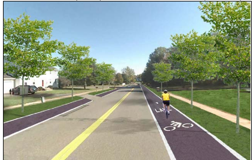
Narrower Pavement (24 Feet) With Street Trees and Bike Lanes (4 Feet Each)
