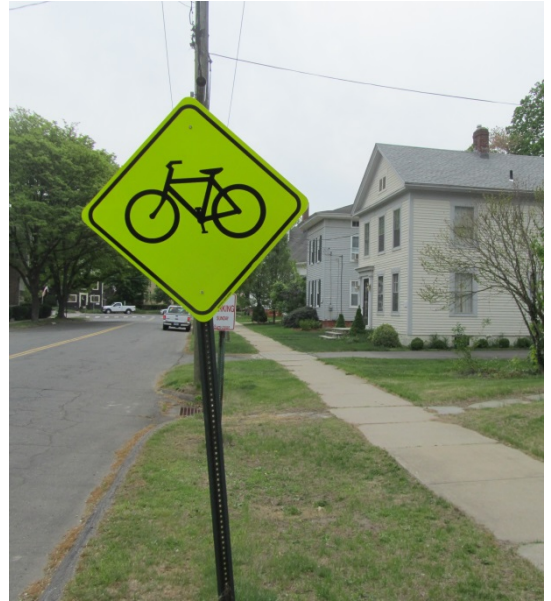
Figure 20: Bicycle Crossing Sign without Edge Line Pavement Markings
